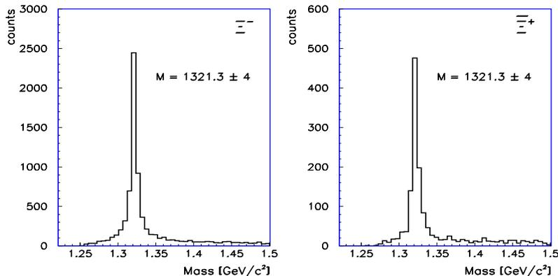
Fig. 1. Invariant mass distributions for  $\Xi^-$  (left) and  $\Xi^+$  (right) from 400 000 central Pb+Pb collisions. In the bin centred on the  $\Xi^-$  mass, the signal-to-noise ratio is better than 10:1.
