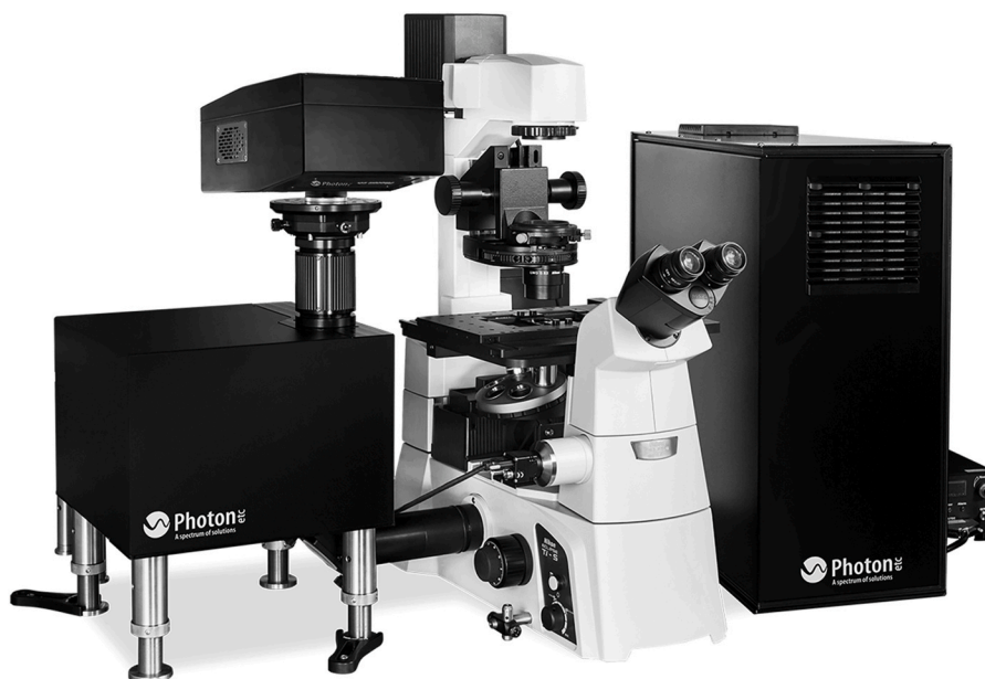
Fig. 2. Hyperspectral fluorescence microscopy system equipped with volume Bragg gratings and an optical microscope.
