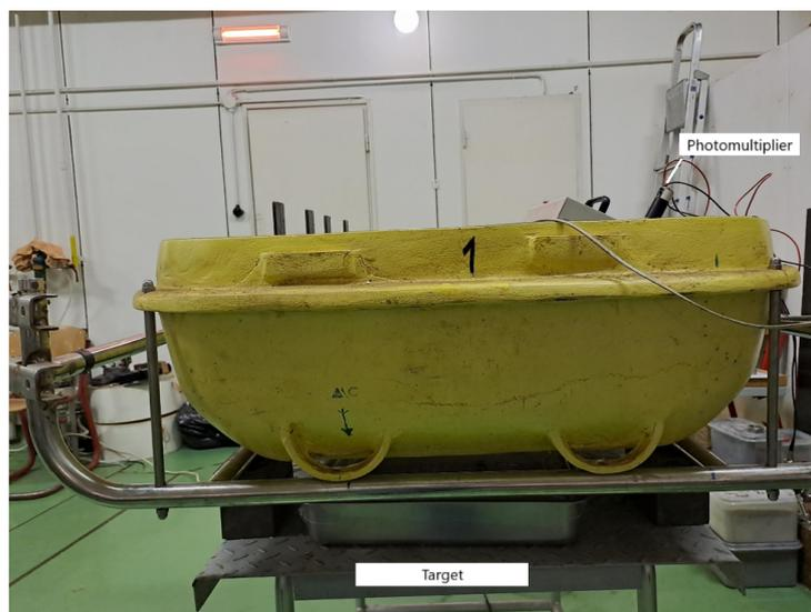
**Figure 3.** Side view of the AAP-based detection setup, showing the Kevlar submarine, target of interest, and the photomultiplier (attached to the alpha detector).
