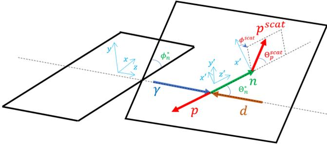
Figure 2: Kinematics of the reaction in the centre of mass system. The z-axis is oriented along the beam, y-axis is perpendicular to the ground; z' axis is oriented along the ejectile neutron direction, y' axis is perpendicular to the reaction plane.
