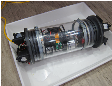
Fig. 28. Submersible ROV developed at the Lancaster University during irradiation tests at the JSI TRIGA reactor.
