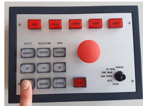
(b) A hardware console was developed for the Research Reactor Simulator.
