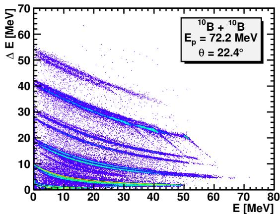
**Figure 1.** An example of the  $\Delta E$ -E spectra for one quadrant of the thin detector and corresponding strips of the DSSSD thick detector in the telescope centered at 22.4°
