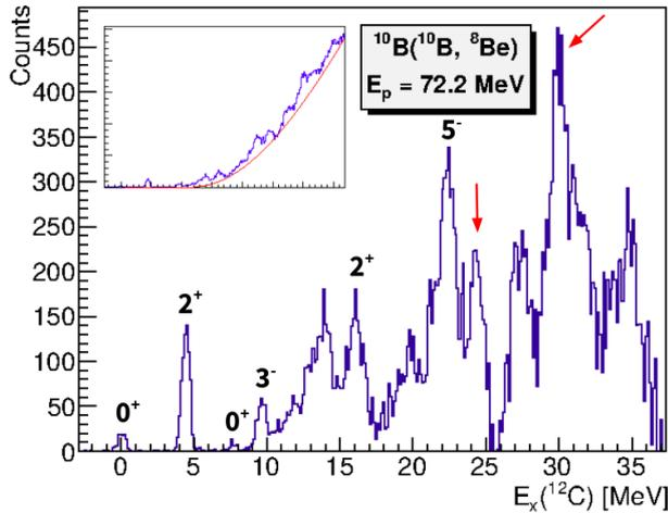
**Figure 3.** The excitation energy spectrum of  $^{12}\text{C}$  for  $2\alpha$  coincidences, obtained with a constraint that the two detected  $\alpha$  particles originate from the  $^8\text{Be}$  ground state. The background-subtracted spectrum is shown in the main panel, while the inset displays the spectrum including the background.
