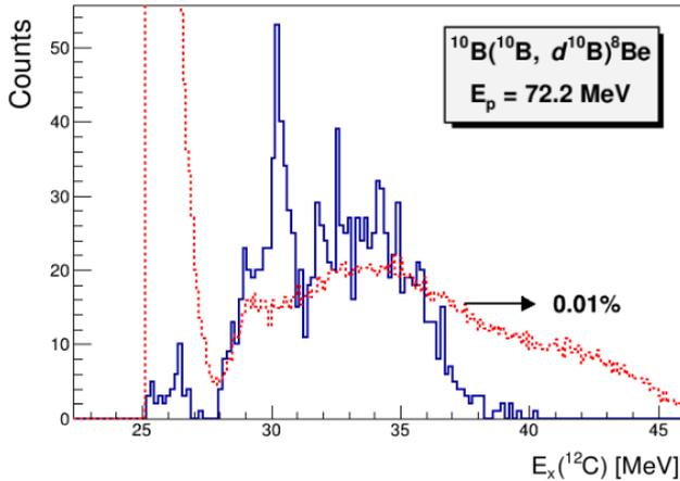
**Figure 5.** The  $^{12}\text{C}$  excitation energy spectrum for the  $d+^{10}\text{B}$  coincidences. The (red) dotted line shows the corresponding Monte Carlo efficiency curve.
