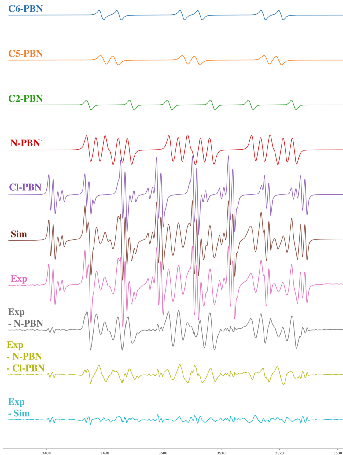
Figure 2. EPR spectra of spin-trapped radical intermediates generated with 370 nm irradiation of N-Cl. The simulated spectra of each radical adduct species are denoted in the spectra as C 6 -PBN, C 5 -PBN, CI-PBN, C 2 -PBN, and N-PBN. Total simulated spectrum is labeled as Sim, while the experimental spectrum is labeled as Exp, with residual signals provided as Exp-N-PBN, Exp-N-PBN-CI-PBN, and Exp-Sim. Line widths measured with EPR and reaction yields were influenced by the effectiveness of air removal using freeze-pump-thaw cycles with backfill of argon or nitrogen gas. Experimental line widths of less than 0.4 G were deemed satisfactory for the optimal resolution of radical adducts. More information on deconvolution and simulation is deposited in the SI.
