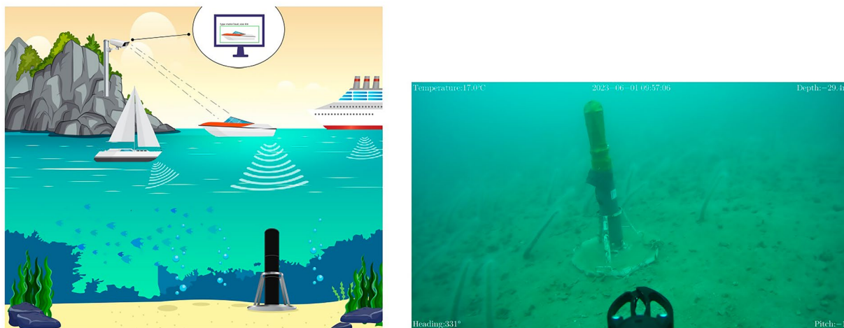
Fig. 1 Setup of the recorder. Left panel: Illustration of the acoustic-optic testbed for quantifying the URN of VOO by using synchronized optical measurements from a shore based camera and an acoustic recorder positioned at the seabed. Right panel: Picture of the underwater acoustic recorder at the deployment site.
