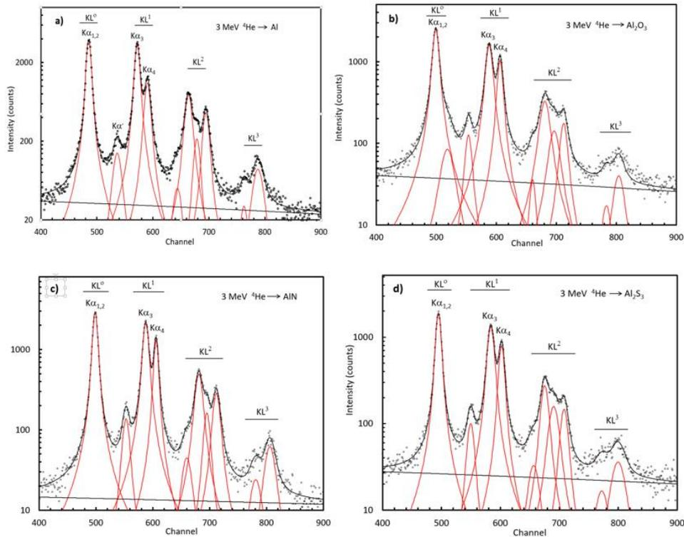
Figure 2. Measured spectra by 3 MeV  $^4\text{He}$  excitation, showing the fitted lines and background models.
