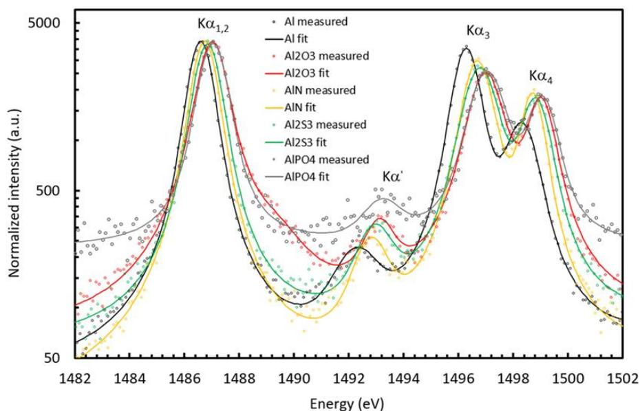
Figure 7. Normalized Al  $KL^0$  and  $KL^1$  regions of the Al spectra from the measured Al compounds excited by 3 MeV He ions.
