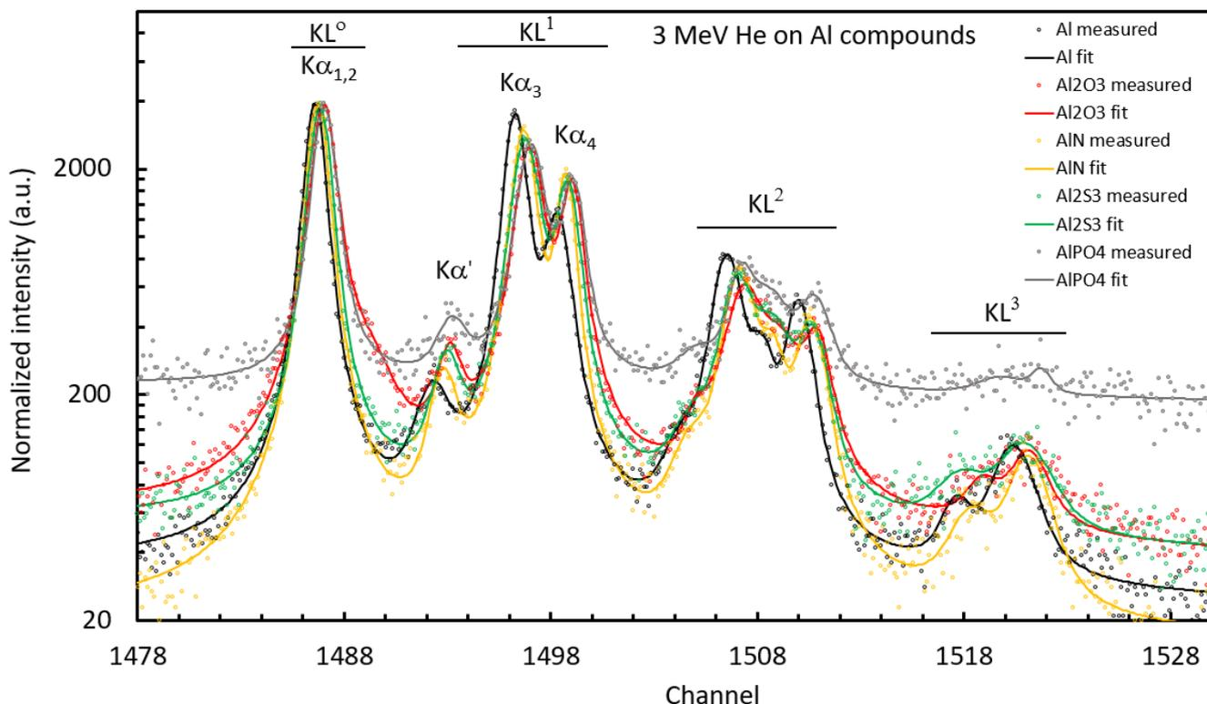
Figure 6. Normalized Al spectra obtained after 3 MeV He excitation.
