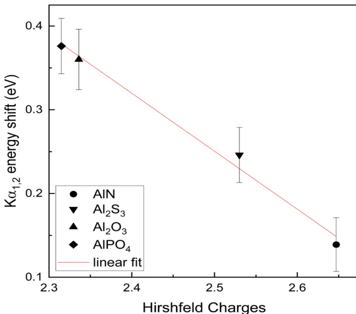
Figure 4. The experimental M1  $K\alpha_{1,2}$  energy shifts vs effective calculated charges on Al atom.
