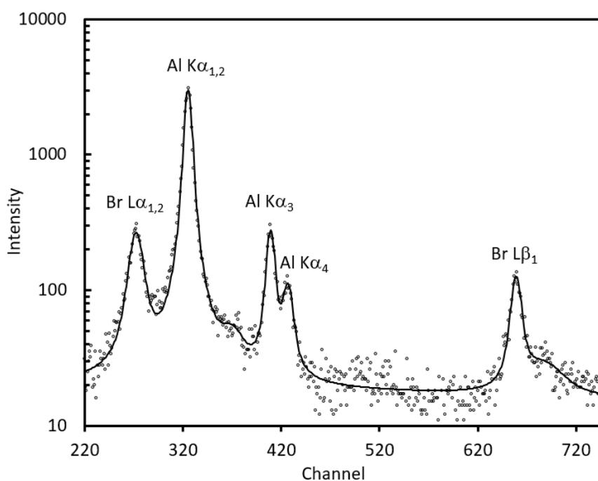
Figure 1. Relevant part of the Al  $K\alpha$  measured spectrum of an Al powder sample mixed with MgBr powder used for energy calibration.
