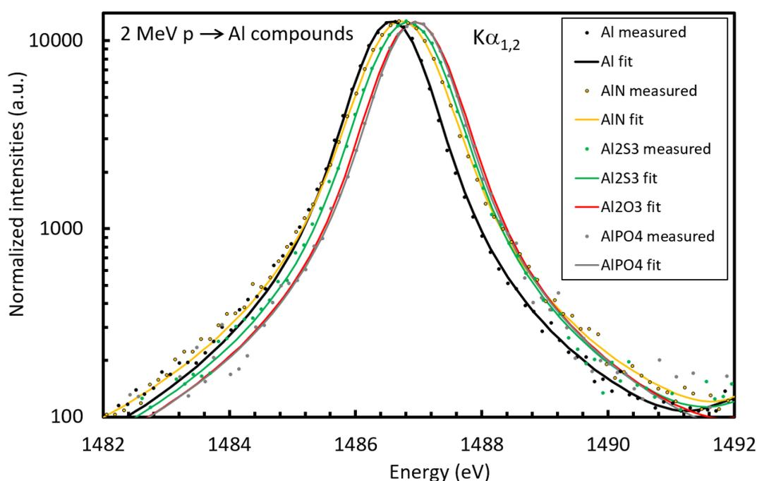
Figure 3. K $\alpha$ <sub>1,2</sub> region of the spectra of all the measured Al compound samples by 2 MeV proton excitation, showing the energy shifts of the Al K $\alpha$ <sub>1,2</sub> line.
