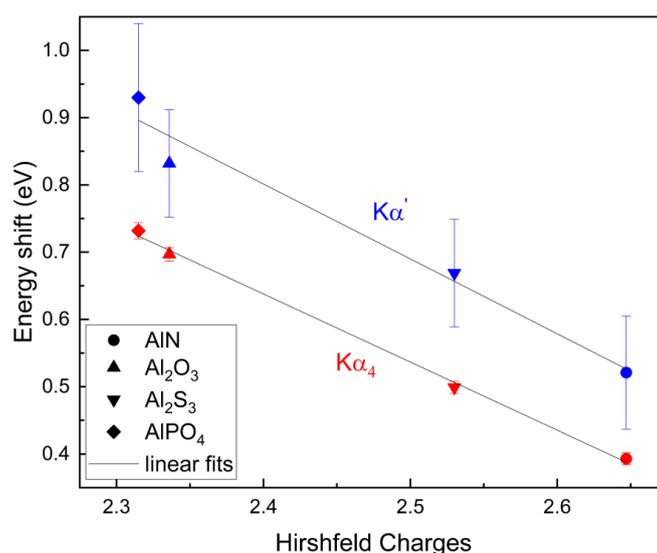
Figure 8: The experimental  $K\alpha'$  and  $K\alpha_4$  energy shifts vs effective calculated charges on Al atom obtained with 3 MeV He excitation.
