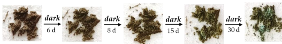
Figure 4. Daylight irradiated compound 1 after being stored in the dark for a different number of days (d).
