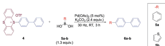
Scheme 2. Mechanochemical Suzuki-Miyaura C-C coupling reaction.
