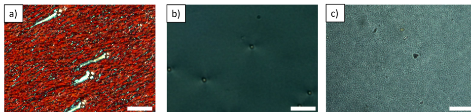
Fig. 5 Optical textures of S-CBCOO7CB in the N^* phase. (a) The texture of the N^* phase at 68 °C obtained on heating in a planar 5 \mu\text{m} cell. (b) The texture of the N^* phase at 57 °C obtained on cooling in a planar 5 \mu\text{m} cell. (c) The texture of the N^* phase at 70 °C obtained on cooling and under mechanical stress. The scale bar is 20 \mu\text{m} .
