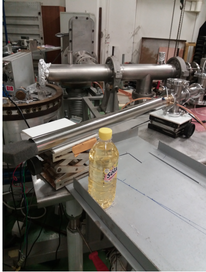
Figure 2: Experimental setup. The PET bottle filled with diesel fuel is placed in one of the four positions for which the time spectra was measured. Instrumentation (scintillators, photomultipliers) is placed inside metallic cylinder.
