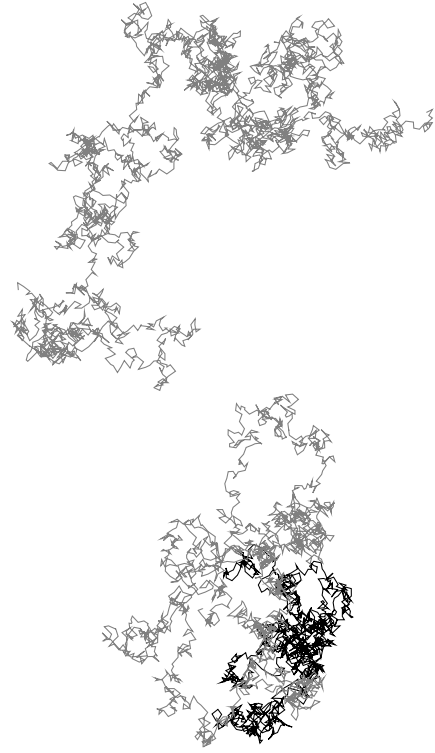
Fig. 2. Schematic BwR representation (3000 steps). A Brownian liquid molecule fluctuates with diffusion coefficient D_1 until time t (gray path). A chain molecule (blackened snapshot) substitutes a portion of this path ( 0 < t' < t ) at a constant diffusivity, similarly to the way the body in Fig. 1 extends within the trajectory, taking up a part of distance to be traveled.
