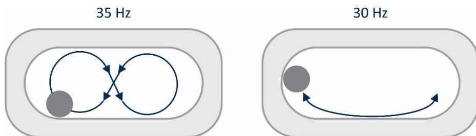
Figure 1: Trajectory of a milling ball ( \varnothing 10 mm) observed at 35 Hz and 30 Hz in a MM500 mixer mill.
