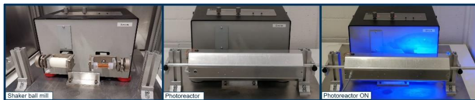
Figure 1 Custom-build photoreactor for mixer mill (IST 500) with UVC LED units for simultaneous photo-mechanochemical reactions.
