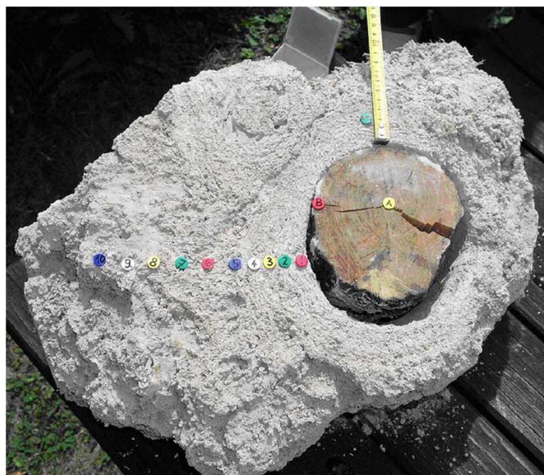
Figure 2. Tufa layer around the wooden pillar taken from the Korana River. Labels from 1 to 10 mark places of tufa sub-sampling. (Letters A and B refer to inner and outer wood layers).
