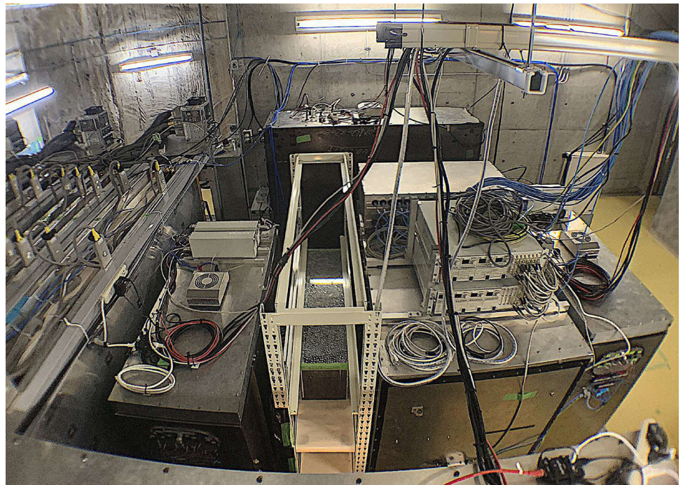
Fig. 176 An NINJA detector includes 9 water-target ECC elements. The NINJA detector is in the centre of the figure. The white rack consists of three tiers, with 3 ECC elements on each tier, for a total of 9 ECC elements in use. An emulsion shifter and a scintillation tracker, which add timing information to emulsion tracks, are placed downstream of ECC elements for \mu identification (by connecting to the Baby-MIND—one of the T2K near detectors)
