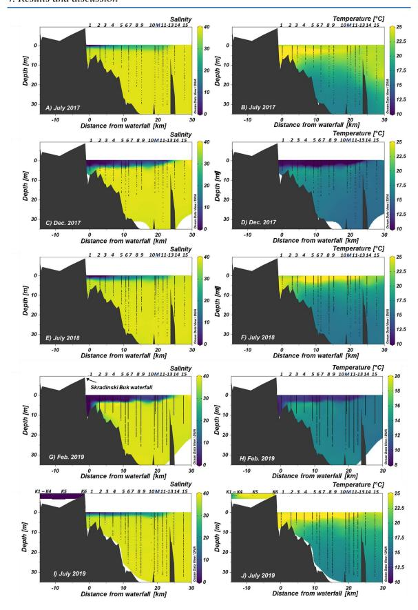
**Figure 4.45.** Vertical distribution of salinity and temperature in the estuary in July 2017, December 2017, July 2018, February 2019 and July 2019. Numbers on the top of the panels indicate the sampling stations and the black dots indicate the sampling points used for the interpolation. Plotted height of the Skradinski Buk waterfall is lower than in reality (46 m) for better representation.
