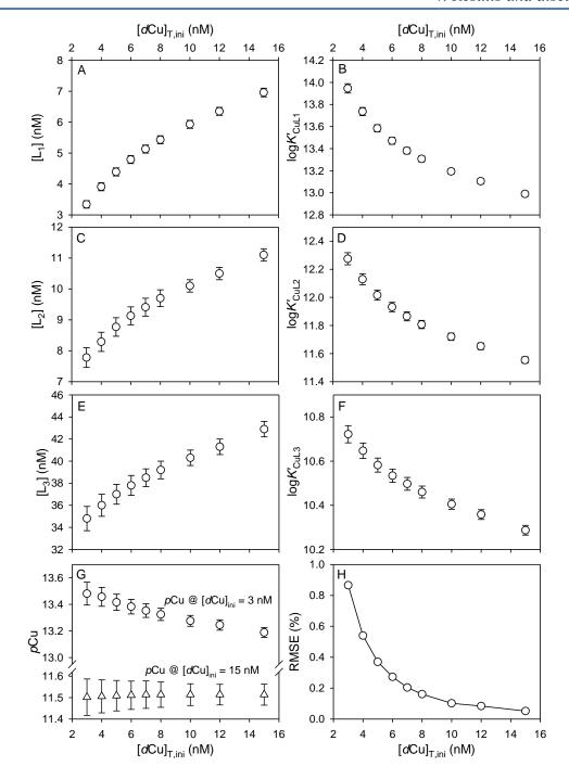
**Figure 4.21.** Complexing parameters ([L<sub>i</sub>] and log  $K'_{\text{CuLi}}$ ), estimated pCu values and RMSE obtained from a simulated NICA-Donnan SMDW complexometric titration at various initial Cu concentrations ([dCu]<sub>T,ini</sub>).
