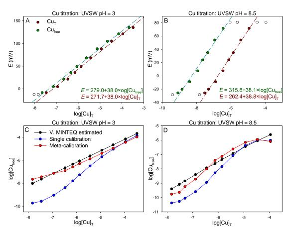
**Figure 4.28. Top:** Electrode response to  $log[Cu]_T$  (brown) and  $log[Cu_{free}]$  (green) change in UVSW at pH = 3 (A) and 8.5 (B). Regression lines are shown as dashed lines and points used for regression are indicated as full circles; equilibrium speciation was calculated using Visual MINTEQ. **Bottom:** Comparison between  $log[Cu_{free}]$  calculated using meta-calibration (red), standard single calibration (blue) and modeled using Visual MINTEQ (black) at pH = 3 (C) and 8.5 (D).
