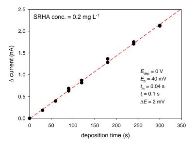
**Figure 4.35.** Dependence of the difference of the signal and the background current on the deposition time obtained in UVSW with addition of 0.2 mg L<sup>-1</sup> SRFA.
