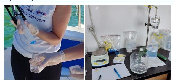
**Figure 3.6.** On board filtering (left) and polycarbonate filtration system for filtration under nitrogen pressure (right).
