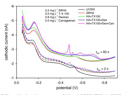
**Figure 4.40.** Differential pulse voltammograms of  $0.2 \text{ mg L}^{-1}$  IHSS SRHA in UVSW, with stepwise addition of other organic compounds (Triton-X-100, dextran and carrageenan) at concentrations indicated in the plot. Full lines correspond to analytical scans performed using 60 s of deposition time, whereas dashed lines are background scans obtained using 2 s deposition time at 0.0 V.
