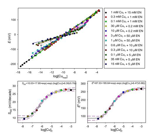
**Figure 4.25. Top:** Electrode response to  $log[Cu_{free}]$  change in 0.5 M NaCl at various  $Cu_T$  concentrations. **Bottom:** Variation of the slope  $S_{ISE}$  (left graph) and intercept  $E^0$  (right graph) vs.  $log[Cu]_T$ . Data were fitted using the Gompertz equation (full lines); dashed lines represent 95% confidence interval.
