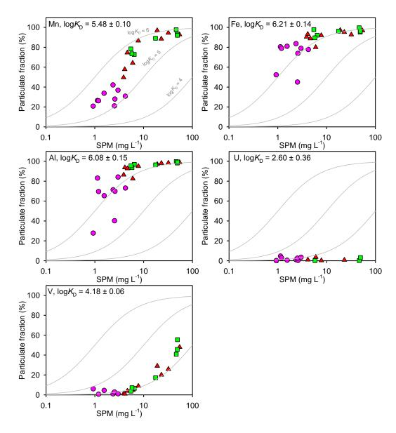
**Figure A5.** Distribution of particulate trace metal fraction in relation to SPM. Grey lines represent theoretical distributions for three different values of  $\log K_D$ , as indicated at the top of the plots.
