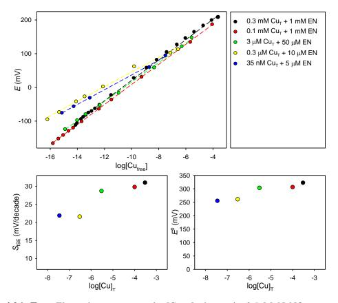
**Figure 4.26. Top:** Electrode response to  $log[Cu_{free}]$  change in 0.5 M NaNO<sub>3</sub> at various  $Cu_T$  concentrations. **Bottom:** Variation of the slope  $S_{ISE}$  (left graph) and intercept  $E^0$  (right graph) vs.  $log[Cu]_T$ .
