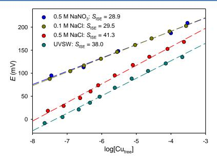
**Figure 4.27.** Electrode response to  $Cu_T$  additions in 0.5 M NaNO<sub>3</sub>, 0.1 and 0.5 M NaCl and UVSW at pH = 3. Regression lines are shown as dashed lines; slope values are expressed in mV/log[ $Cu_{free}$ ]; [ $Cu_{free}$ ] was calculated using Visual MINTEQ.
