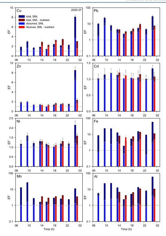
**Figure 4.62.** Enrichment factors (EF) for dissolved and total concentrations of selected trace elements (as indicated in figure) obtained in the SML and SML-bubbled samples collected in July 2020. Horizontal dashed line indicates the unity with the ULW.
