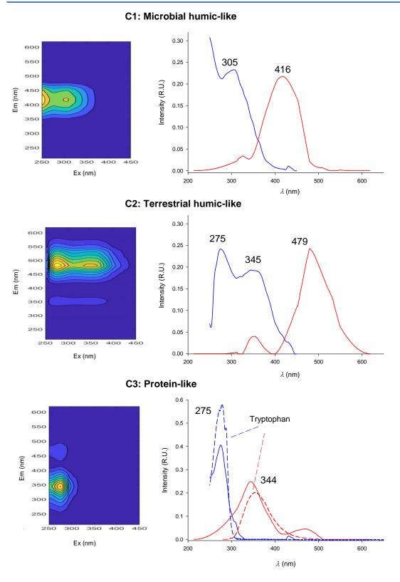
**Figure A1.** Excitation (in blue) and emission (in red) spectra and 3D view of 3 PARAFAC components validated in Dataset 1 and Dataset 2. The spectra of protein-like component are overlapped to Tryptophan standard (dashed lines).
