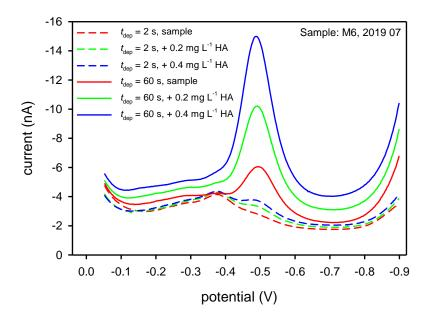
**Figure 4.43**. Typical voltammograms of the HS determination in real estuarine sample (M6, 2019 07) using Mo-HS method. Solid lines represent analytical signals obtained at 60 s deposition time, without and with two additions of HA (IHSS SRHA) as identified in the plot. Dashed lines represent background scans obtained at 2 s of deposition time at -0.2 V. The electrochemical parameters are given in Section 3.5.1.3, **Table 3.6**.
