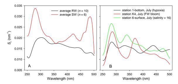
**Figure 4.53.** A) Spectral slope curves calculated on averaged absorption spectra of freshwater and seawater samples and B) spectral slope curves calculated on absorption spectra of three selected samples.
