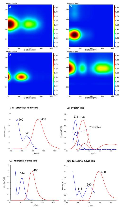
**Figure A6.** 3D view (top 4 plots) and excitation (in blue) and emission (in red) spectra (bottom 4 plots) of the 4 PARAFAC components validated in the SML Dataset. The spectra of protein-like component are overlapped to those of Tryptophan standard (dashed lines)
