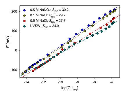
**Figure 4.23.** Electrode response to  $log[Cu_{free}]$  increase in 0.5 M NaNO<sub>3</sub>, 0.1 or 0.5 M NaCl and UVSW in presence of 0.3 mM  $Cu_T$  and 1 mM EN. Calibration lines are shown as dashed lines; slope values ( $S_{ISE}$ ) are expressed in mV/decade;  $log[Cu_{free}]$  was varied by adjusting the pH based on equilibrium speciation calculated by Visual MINTEQ.
