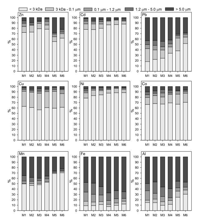
**Figure 4.70.** Average percentages of studied trace metals in each size fraction (as indicated in the figure) at each depth (M1 - M6).
