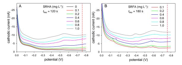
**Figure 4.37.** Typical differential pulse voltammograms obtained in UWSV at increasing concentrations of IHSS SRHA (A) and SRFA (B) as indicated in the plots. The electrochemical parameters are given in Section 3.5.1.3, **Table 3.6**. Vertical red dashed lines represent a potential at which the differential current (the current relative to a background scan at 2 s deposition time) was determined and used as an analytical measure for the determination of unknown concentration of HS.
