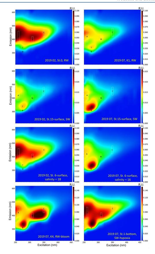
**Figure 4.52** EEMs of selected samples. The positions of peaks A, M, C, B and T as named by Coble (1996) are reported on each EEM.
