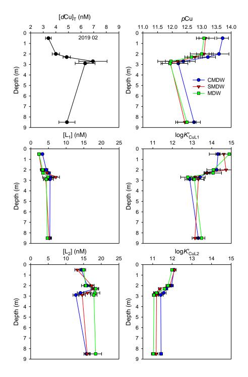
**Figure 4.19.** Comparison of the results obtained by MDW, SMDW and CMDW approaches on samples from vertical profile of the Krka River estuary sampled on February 2019: (A) ambient dissolved Cu concentrations, (B) ambient pCu estimates, (C) [L<sub>1</sub>], (D)  $\log K'_{\text{CuL1}}$ , I [L<sub>2</sub>] and (F)  $\log K'_{\text{CuL2}}$ .
