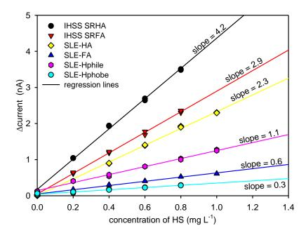
**Figure 4.38.** Calibration plots for different types of model organic matter (indicated in plot) obtained with 60 s deposition time at 0.0 V using the new PB-HS method.  $\Delta$  current is an average of the current from -0.75 to -0.80 V relative to a background scan at 2 s deposition time. The electrochemical parameters are given in Section 3.5.1.3, **Table 3.6**.
