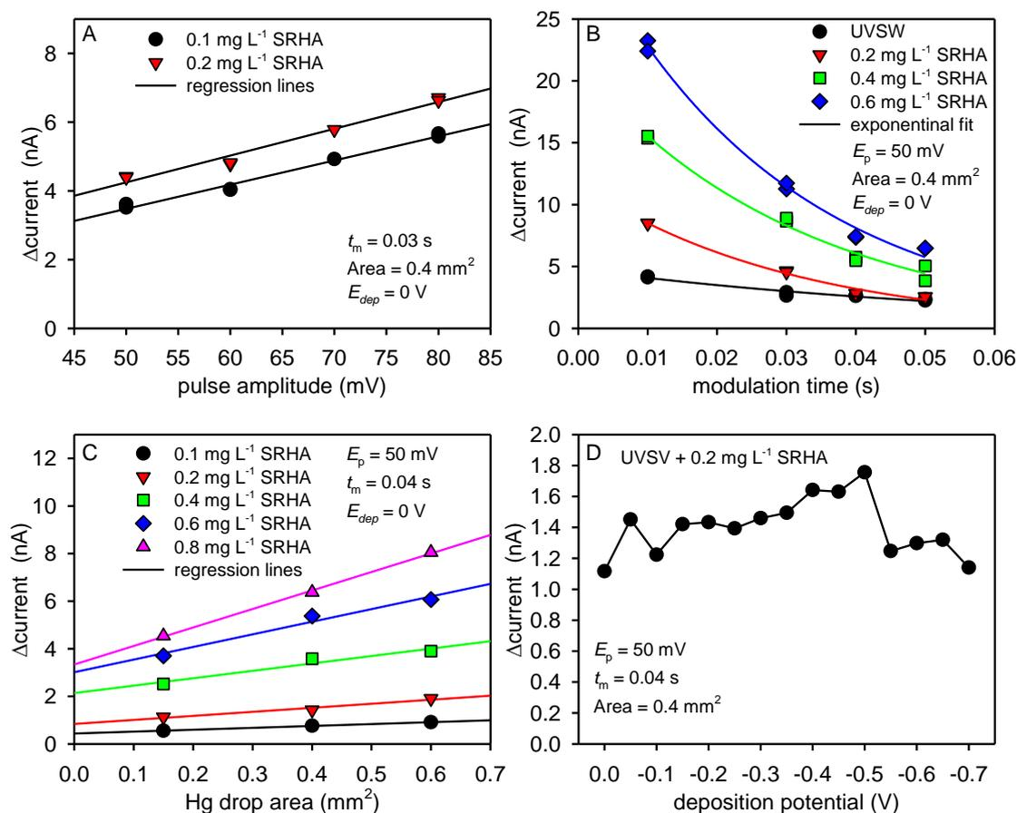
**Figure 4.36.** Impact of A) pulse amplitude ( $E_p$ ), B) modulation time ( $t_m$ ), C) Hg drop area and D) deposition potential ( $E_{dep}$ ) on the capacitive current.  $\Delta$  current is an average of the current from -0.75 to -0.80 V relative to a background scan at 2 s deposition time. Fixed parameters are indicated in each panel. The deposition time was 120 s and interval time of 0.1 s and step potential of 2 mV were used.
