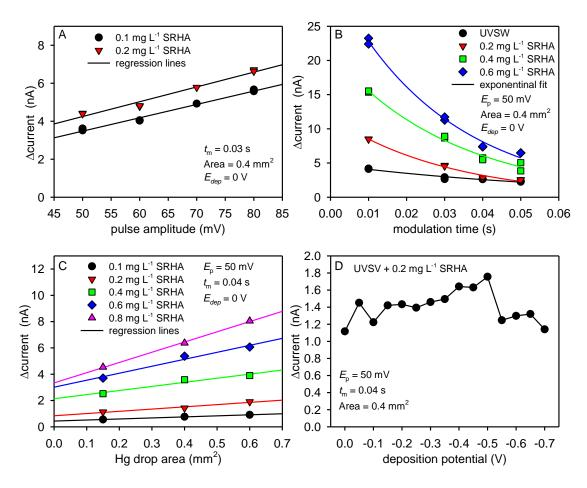
**Figure 4.36.** Impact of A) pulse amplitude ( $E_p$ ), B) modulation time ( $t_m$ ), C) Hg drop area and D) deposition potential ( $E_{dep}$ ) on the capacitive current.  $\triangle$  current is an average of the current from -0.75 to -0.80 V relative to a background scan at 2 s deposition time. Fixed parameters are indicated in each panel. The deposition time was 120 s and interval time of 0.1 s and step potential of 2 mV were used.
