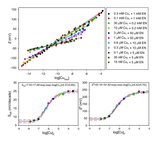
**Figure 4.24 Top:** Electrode response to  $log[Cu_{free}]$  change in UVSW at various  $Cu_T$  concentrations. **Bottom:** Variation of the slope  $S_{ISE}$  (left graph) and intercept  $E^0$  (right graph) vs.  $log[Cu]_T$ . Data were fitted using the Gompertz equation (full lines); dashed lines represent 95% confidence interval.
