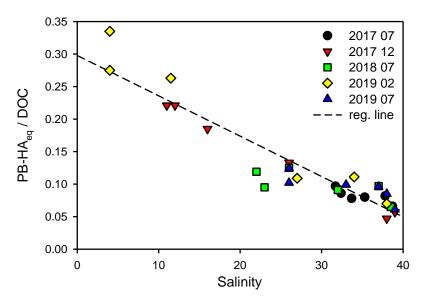
**Figure 4.41**. Distribution of DOC-normalized concentration of  $HA_{eq}$  in the salinity gradient at station M (Martinska Marine station) obtained using a new PB-HS method for samples collected over different sampling campaigns.
