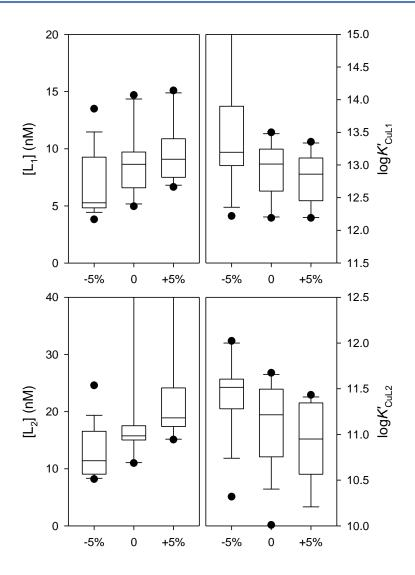
**Figure 4.22.** 'Box-plots' of Cu complexing parameters (sample from 2.5 m depth, M4 in December 2017) obtained by combining different experimental conditions, and data treatment routines for both voltammograms and titration curves. Additional tests included the influence of  $\pm$  5% change in applied sensitivity.
