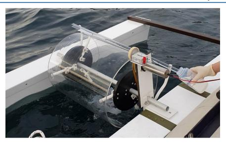
**Figure 3.5.** Sampling of the sea surface microlayer by a drum sampler.
