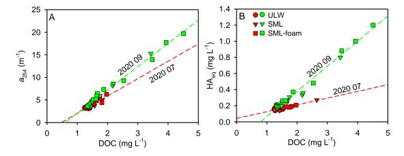
**Figure 4.65.** Dependence of absorption coefficient at 254 nm ( $a_{254}$ ) (A) and humic acid equivalent concentration (HA<sub>eq</sub>) (B) on DOC concentration for the two sampling periods. All measurement data are used to plot relationships. Dashed lines represent the regression lines.
