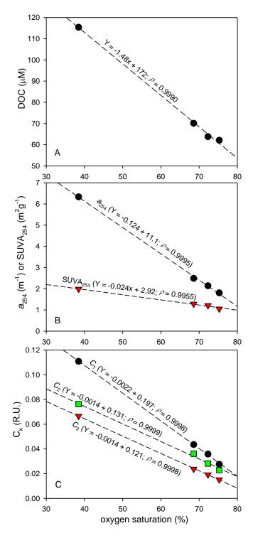
**Figure 4.51.** Relationship in the hypoxic waters (samples with oxygen saturation < 75%) between oxygen saturation and A) DOC, B) absorption coefficient at 254 nm ( $a_{254}$ ) and SUVA<sub>254</sub> and C) 3 PARAFAC components validated in Dataset 1. Regression lines are plotted as dashed lines.
