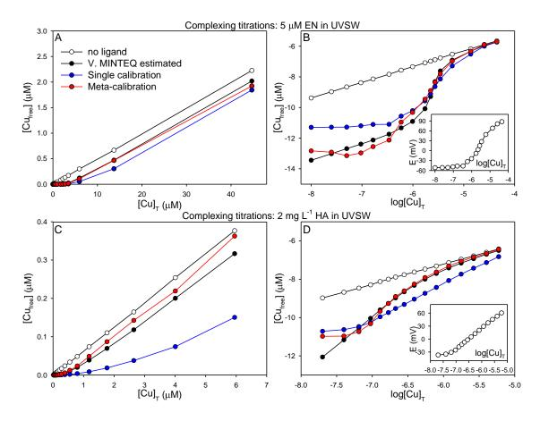
**Figure 4.30.** Complexometric titrations in UVSW comprising 5  $\mu$ M EN (A, B) and 2 mg L<sup>-1</sup> HA (C, D): comparison between [Cu<sub>free</sub>] calculated using meta-calibration approach (red), single calibration approach (blue) and modeled using Visual MINTEQ with (black) and without (white) organic ligands in the solution, in linear (A, C) and logarithmic scale (B, D). Insets: Corresponding E-log[Cu]<sub>T</sub> curves.
