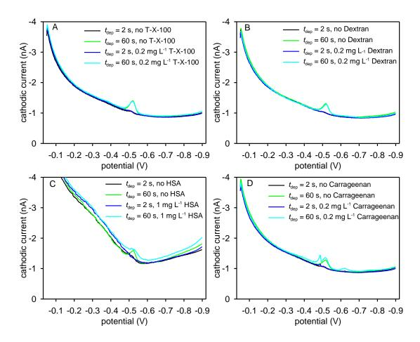
**Figure 4.39.** Differential pulse voltammograms obtained in UVSW without and with addition of Triton-X-100 (A), dextran (B), carrageenan (C) and human serum albumin (HSA) (D) at concentrations indicated in plots. The analytical scans were performed using 60 s deposition time, whereas background scans were obtained with 2 s deposition time at 0.0 V.
