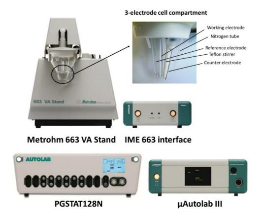
Figure 3.7. Metrohm-Autolab instruments and 3-electrode cell system used in this work.
