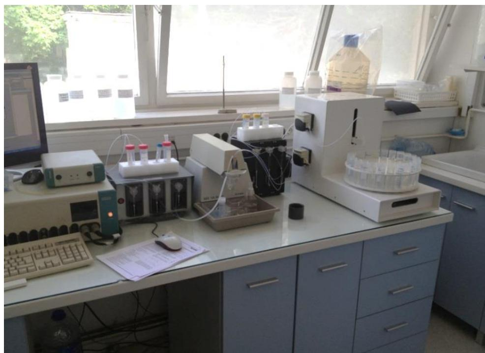
**Figure 3.14.** Automated voltammetric system for trace metals analysis
