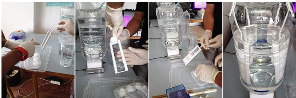
**Figure 3.16.** Set up for DGT “diffusion coefficient” experiment
