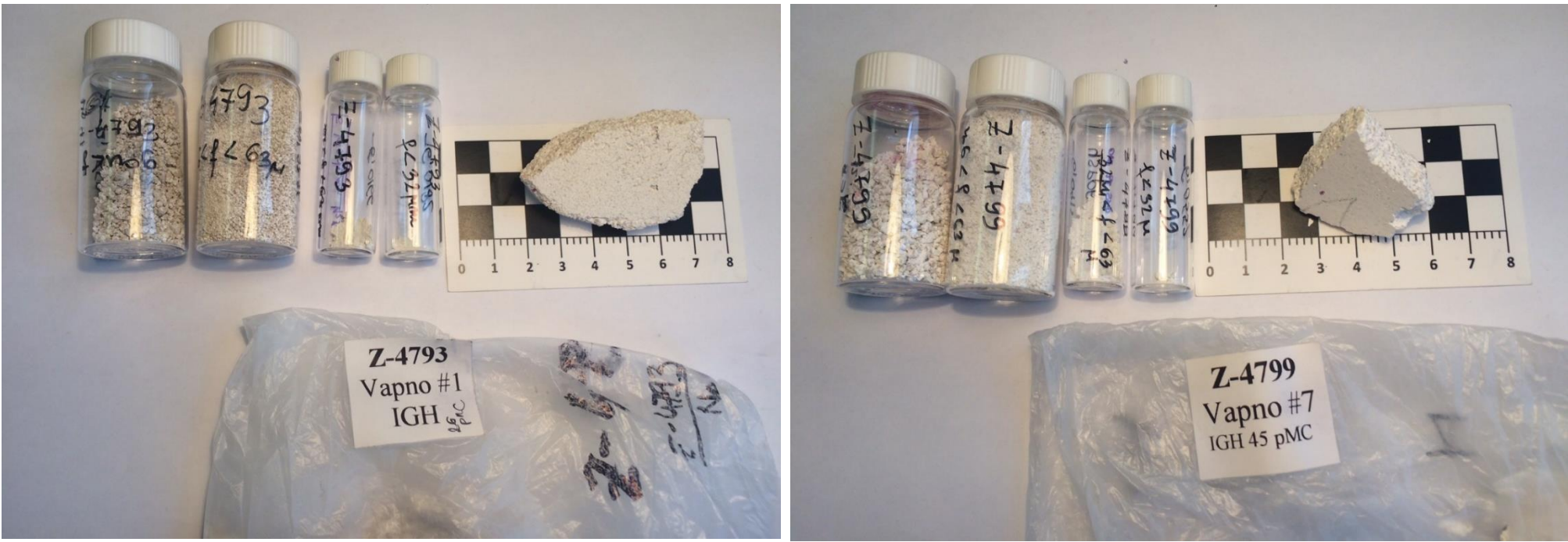
Mortar samples Vapno #1 and Vapno #7 vials with particle fractions: >3.35 mm, 3.35 mm – 63 μm , 63 – 38 μm and < 38 μm, and pieces of hardened mortars
