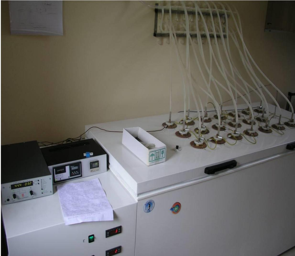
The main part of the system of electrolytic enrichment consists of 20 cells of 500 mL volume placed in a refrigerator that cools the cells and keeps them at 2–5 °C to prevent the loss of tritiated water molecules by evaporation during the electrolysis.
