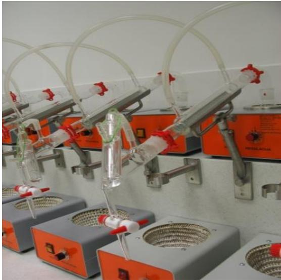
Each enrichment run contains 15 unknown samples, 3 spike waters (water of known tritium activity concentration) used for monitoring the electrolysis performances and 2 tritium-free (“dead water”) samples used for system control.
