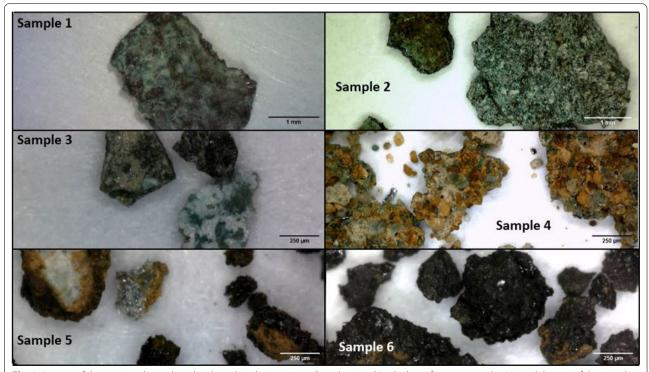
Fig. 2 Images of the examined samples taken by a digital microscope: Samples 1 and 2 which are fragments under 60x and the rest of the samples under 240x magnification
