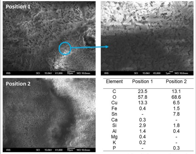
Fig. 5 SEM image of two different positions on Sample 3 and elemental composition in atomic-% obtained on the two positions by point analysis
