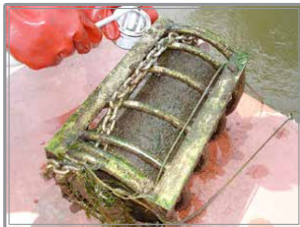
Fig. 2. Semi permeable membrane device used in monitoring Sava river.
