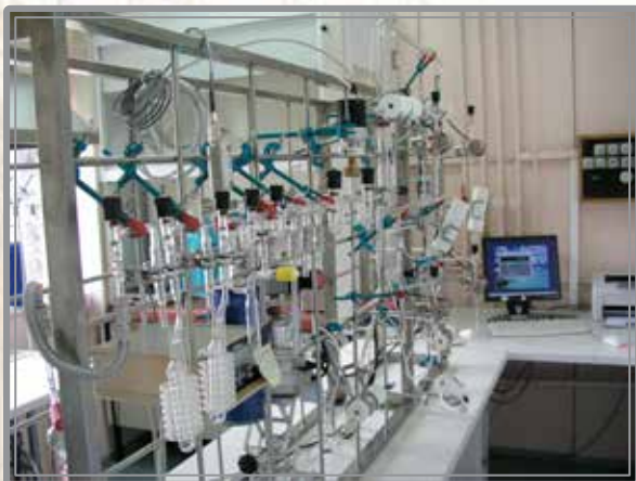
Fig. 6 Vacuum line for preparation of graphite for ^{14}\text{C} AMS measurement technique.
