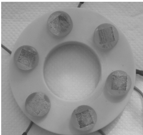
Figure 1. Parallel connection of six electrodes for the electrochemical patination.
