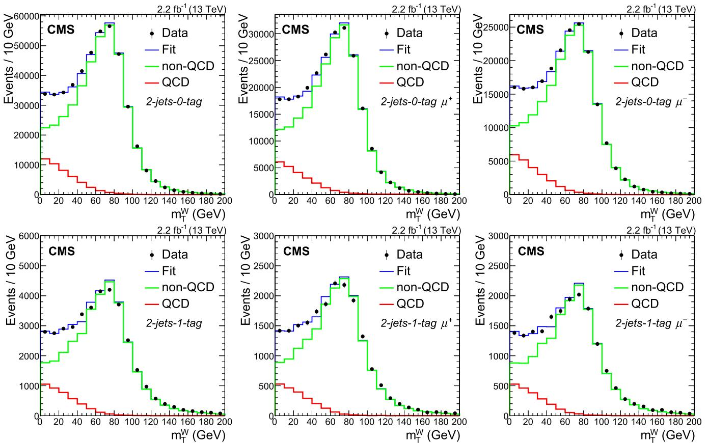
**Fig. 2.** Fit to the  $m_T^W$  distributions in the 2-jets-0-tag sample (upper row) and the 2-jets-1-tag sample (lower row) for all events (left), for positively charged muons only (middle), and for negatively charged muons only (right). The QCD fit template is derived from a sideband region in data. Only statistical uncertainties are taken into account in the fit.
