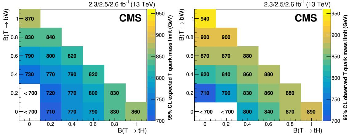
**Figure 14.** The expected (left) and observed (right) at 95% CL lower limits (Bayesian) on the T quark mass for a variety of  $T \rightarrow tH$  and  $T \rightarrow bW$  branching fraction combinations, indicated by the coordinates at the center of each box, after combining the boosted W and boosted H channels. A limit of  $< 700$  GeV indicates that this search is not sensitive to T quark decays with that branching fraction combination.
