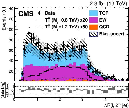
**Figure 5.** Distribution of  $\Delta R(\ell, j_2)$  in the boosted W channel after all selection requirements except for  $\Delta R(\ell, j_2) > 1$ . Also shown are the distributions of  $T\bar{T}$  signal events with T quark masses of 0.8 and 1.2 TeV, scaled by factors of 20 and 60, respectively. The uncertainty in the background includes the statistical and systematic uncertainties described in section 7.
