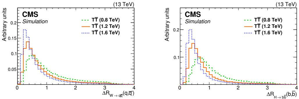
**Figure 2.** Angular separations  $\Delta R$  between the products of simulated  $W \rightarrow q\bar{q}'$  (left) and  $H \rightarrow b\bar{b}'$  (right) decay processes for three different mass points of the  $T$  quark. Even for the lowest mass point shown, the final state particles are typically emitted with a separation of  $\Delta R < 0.8$  and are merged into an AK8 jet.
