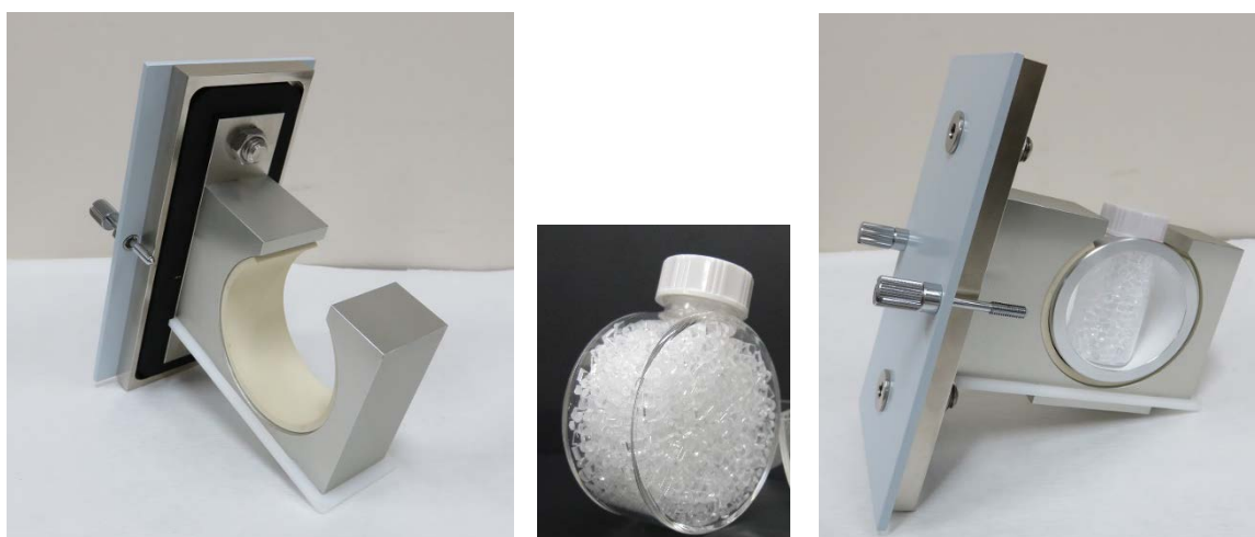
Fig. 1 Photos of the insert part of the plastic scintillator device of PSC-va with PS-pellets.
