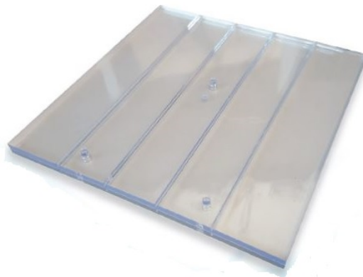
Fig. 1. Illustration of an injection-moulded plastic scintillator tile.
