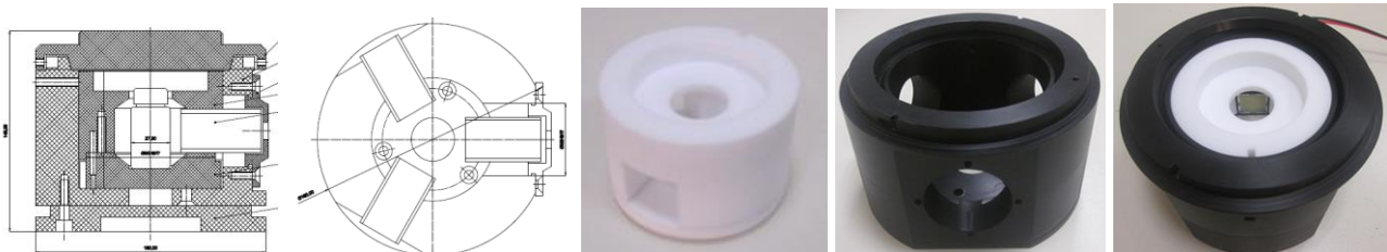
Fig. 1. Description of the TDCR-SU system. Left to right: Cross-sectional front and top views of the counter; the optical chamber; the housing and the counter with a mounted PMT.
