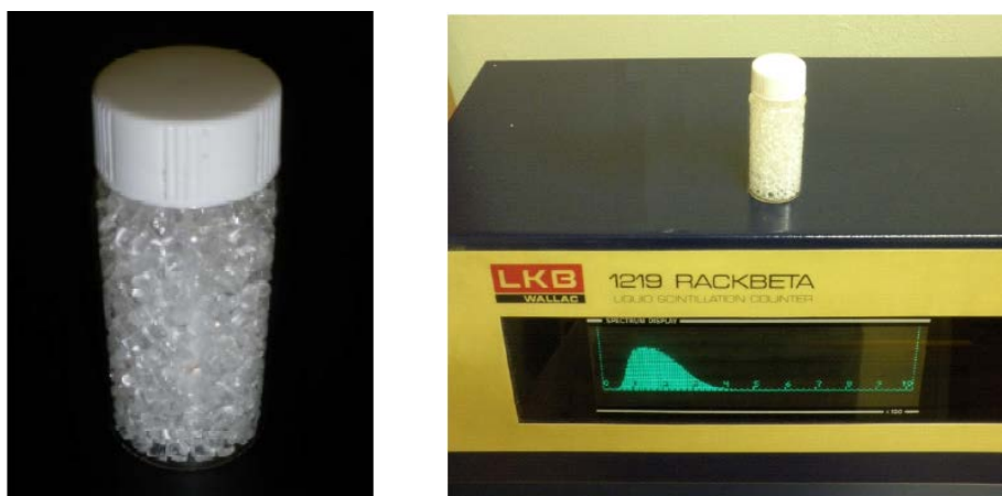
Figure 1. A 20 ml high performance glass vial fully filled with 15g polycarbonate pellets (left). The vial and the RackBeta LS analyzer in the course of measurement of a plastic PVE vial filled with 15g of polycarbonate pellets exposed to ^{222}\text{Rn} (right).
