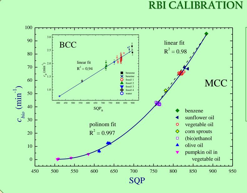
RBI calibration technique uses liquids of different colours to construct modern and background calibration curves, MCC and BCC, respectively, by measuring count rates and SQP(E) values of various modern and fossil liquids.
