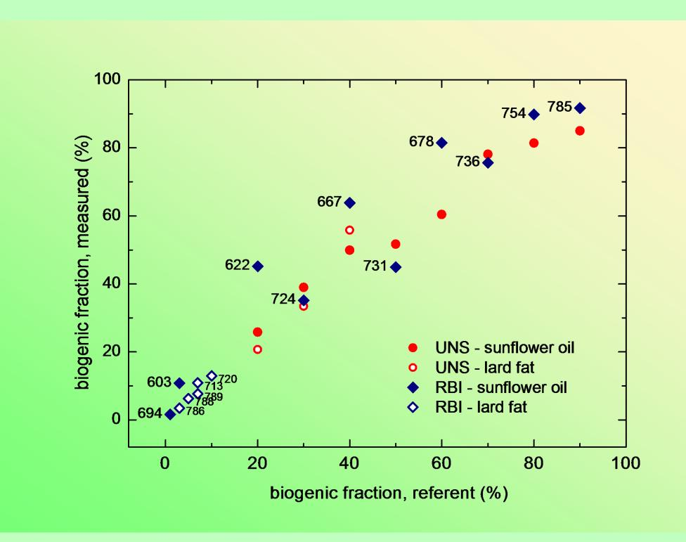
Correlation between the biogenic fraction measured at RBI and UNS and the referent biogenic fraction. The numbers represent the SQP(E) values of the corresponding samples measured at RBI.
