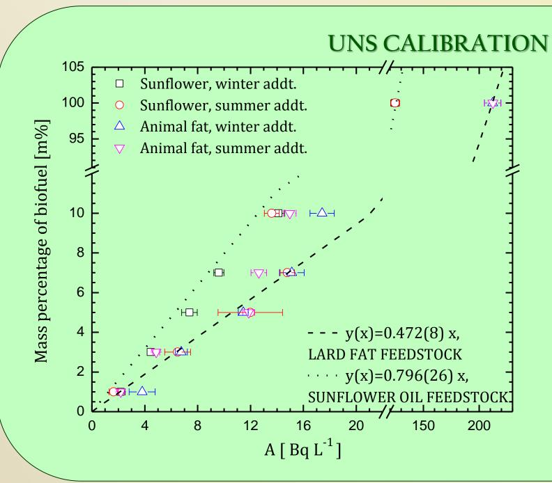
UNS performed a two-step method for calibration. Two-step calibration procedure assumes application of previously established efficiency vs. SQP(E) correlation, followed with activity concentration vs. biogenic content in fuel.
