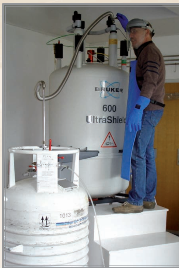
Figure 1. Helium refilling of the 14 T magnet (Bruker 600 MHz).
