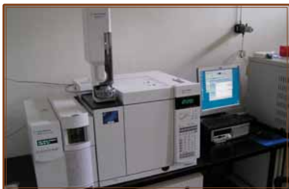
Figure 1. Single quadrupole GC/MS system installed in the Laboratory for Biogeochemistry of Organic Compounds.
