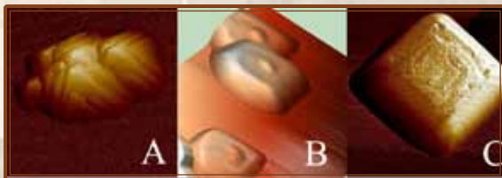
Figure 1. AFM image of the features appearing in the solid phase of the reaction mixture (initially aluminosilicate hydrogel) during its hydrothermal treatment at 80 °C for (A) 30 min ("pyramidal-shaped" particles which represent the first visualization of zeolite nuclei), (B) 90 min (zeolite A microcrystals formed by the growth of nuclei: top of nucleus can be observed near the centre of the 001 crystal faces of each microcrystal) and (C) 240 min (final product; zeolite A crystals with typical growing terraces).
