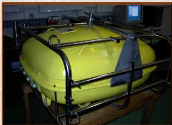
Figure 6. The prototype of the underwater system "Surveyor" containing neutron generator.
