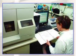
Figure 3. The Abi Prism 310 Genetic Analyzer
