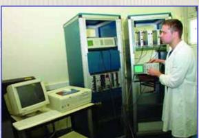
Figure 4. Moessbauer spectrometer for materials research
