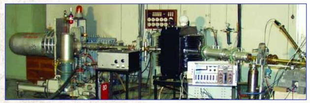
**Figure 5.** The recently refurbished low-energy accelerator which delivers energetic neutrons via the deuteron produced in tritium fusion has become known as the neutron generator. It is used in applied research.
