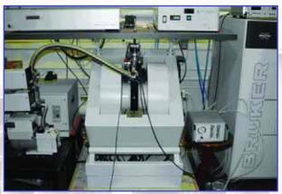
Figure 2. Electron Paramagnetic Resonance spectrometer (FT/CW EPR) working with the pulse and continuous microwave source in a wide temperature range (4K-300K)
