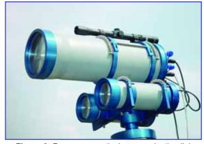
Figure 3. Free space optical communication link developed in CIR in cooperation with LAIR (project HITRA)
