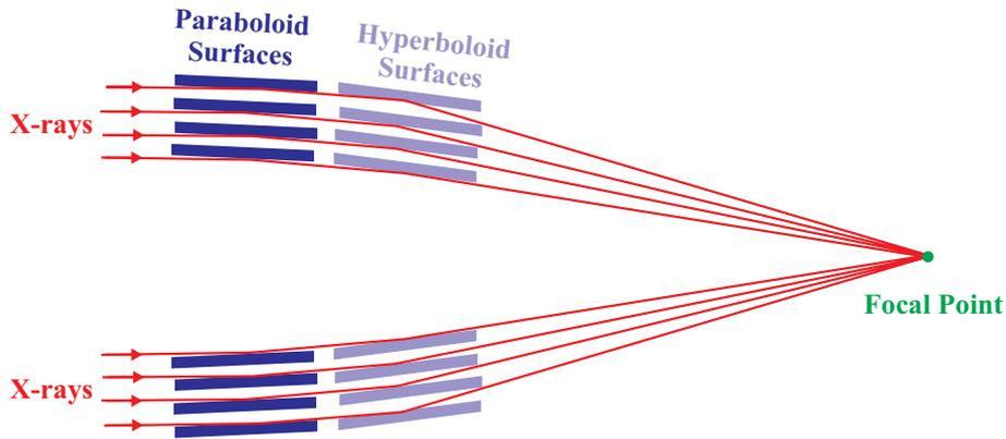
**Figure 1.4:** X-ray telescopes must be very different from optical telescopes. X-ray photons can penetrate into a mirror hence mirror should be shaped and aligned nearly parallel to incoming X-rays. Therefore, X-rays hit the mirrors at a grazing angle.
