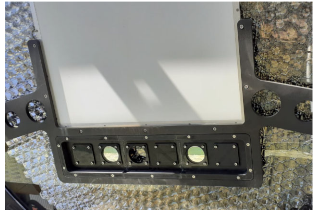
Figure 4. Filter holder of the MAGIC telescopes below the white target, with room for six filters. At the time the picture was taken only two filters were installed, one of the holes was left open and three holes were closed with a plastic cap. Behind the filter holder and the diffusive white target one can see the hexagonal light concentrators (Winston Cones) right in front of the PMTs.
