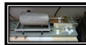
Permittivity vs T (Tc measurement)
