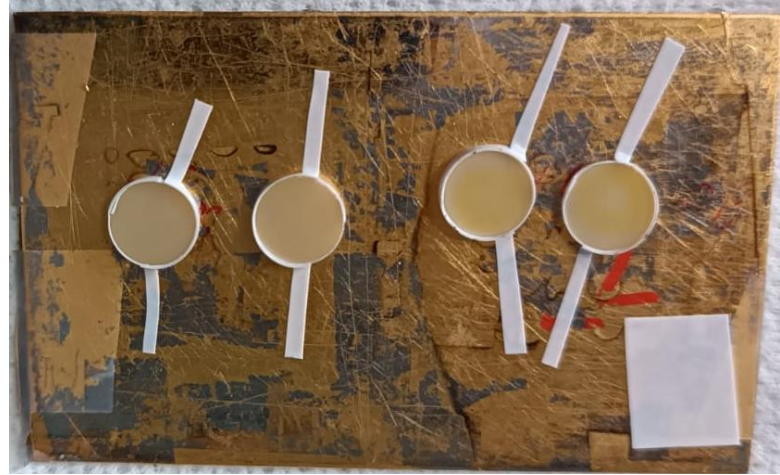
fixing on the sputtering magnetic holder
